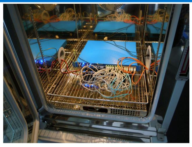
Managed to ensure error-free operation in -15C/+75C environment, and in presence of EMI fields of up to 180V/m. Yeah!
