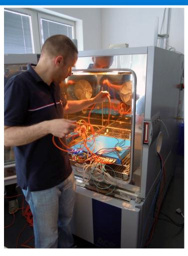
Managed to ensure error-free operation in -15C/+75C environment, and in presence of EMI fields of up to 180V/m. Yeah!
